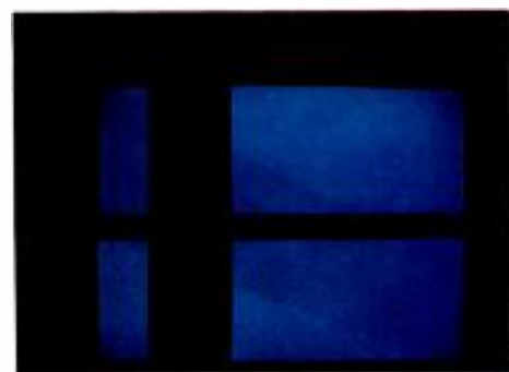
Use of the cross-pulse mode allows the structure of the blanking interval contents to be seen.
